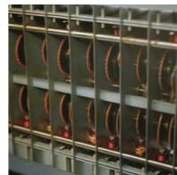
Detail of the original tone wheel components
