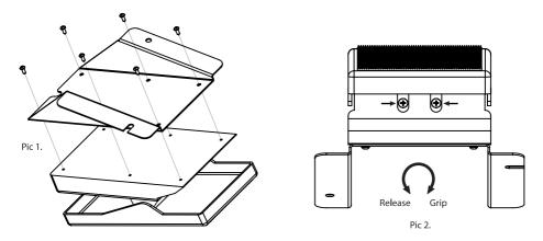
3. Mount the swell pedal assembly on top of the pedal board and tighten the star knobs.
