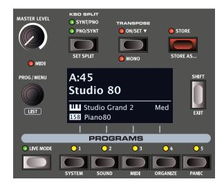
The Program section provides access to performance functions such as loading and storing programs, access to Live programs, keyboard split functionality and more. This is also where menus containing *System*, *Sound* and *MIDI* settings are found. The menus and their settings are covered in a separate chapter, starting on page 22.
