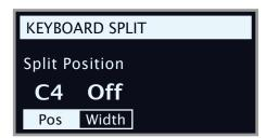
4) There are two settings for the split point; position and width. Make sure that the Position setting is focused (by pressing the Pos soft button) and set the split point to C4 using the dial.
