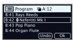
(5) Select the *destination* location for the operation, using the dial and press **Ok**. Pressing **Undo** will instead cancel the operation.
