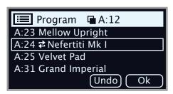
3 Use the dial to select the destination and press **Ok** to complete the Swap operation. Pressing **Undo** will instead cancel the operation.
