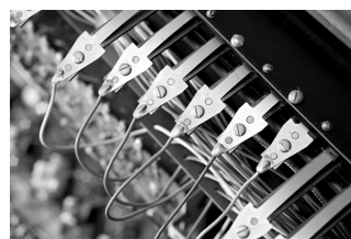
This is the inside of the drawbars. Underneath, you can vaguely see some of the coils for the magnetic pick-ups.
