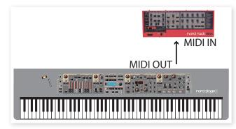
It is best to consider the Extern A/B sections, as simply another pair of onboard instruments, just like the Organ/Piano/Synth sections. Assigning zones/layers, enabling pitch stick and sustain pedal response, etc., are all done in exactly the same manner as with any of those other instrument sections.
