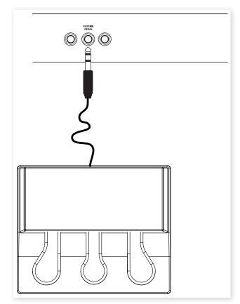
Connect the ¼" stereo connector from the Nord Triple Pedal to the Sustain Pedal connector on the Nord Stage 2.
