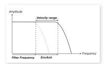
Frequencies above the Filter Frequency setting will be attenuated, frequencies below will not be affected.
