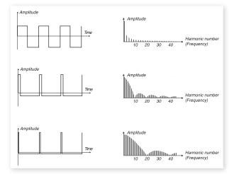
The Shape knob controls the pulse width of the pulse wave, from 50% (square wave) to 1% if the ShP wave is selected. You can modulate the Shape using Morph (see page 19), with the LFO or the Mod Envelope. This waveform is suitable for many type of sounds and has a more "hollow" character than the Sawtooth wave.
