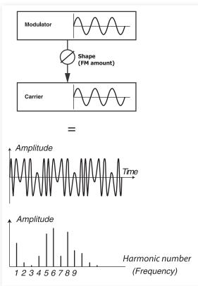
The image above shows a 2 Operator FM-Synthesis setup, and the resulting waveform using a fairly high FM amount setting.
