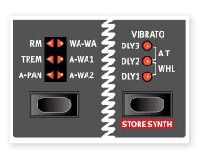
Selector buttons are used to select one setting in an array. They have a set of round or triangular LEDs to indicate the current setting. Press the button several times to cycle through the possible options.
