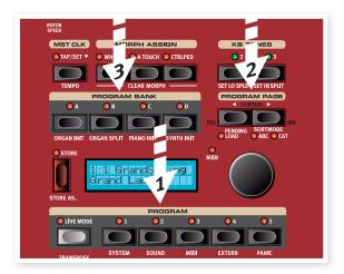
Press and hold either of the Program Page buttons to continuously scroll through the Pages.
