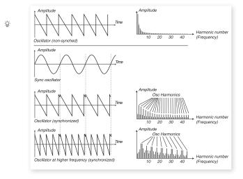
When using Oscillator Sync, it can be very useful to have the Shape amount(s) modulated from any of the Morph assign sources, or by the Modulation Envelope. This will generate a signal with continuously varied harmonic content.
