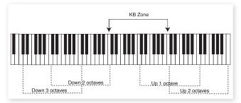
In the illustration above, a piano has been assigned to play in a KB Zone stretching from middle C4 to C6. Without Octave Shift, the actual note range that will be played will be the same as the set zone. The dotted lines show which note range will be played in the set zone when using Octave Shift. In this example you can transpose the piano up or down two octaves to play any two octave note range from the KB zone.
