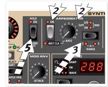
(4) Hold Shift and press the Arpeggiator button repeatedly to select a range.
