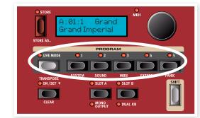
Nord's Live Mode feature provides you with five temporary program buffers, any one of which will automatically save program edits for you on the fly without having to perform a Store operation.
