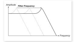
The Filter Frequency is used for setting the cutoff frequency point where in the frequency range the filter begins to process frequencies. This parameter can be Morph controlled.
