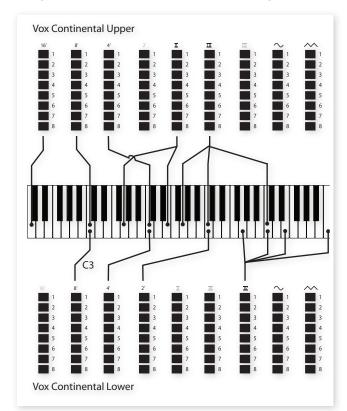
The two drawbars on the right control the sum of all partials in the form of a filtered signal sounding soft and dark, and an unfiltered signal sounding bright and intense.
