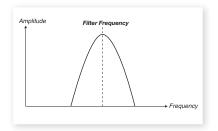
A bandpass filter allows frequencies close the Filter Frequency setting to pass, while frequencies above and below the cutoff will be attenuated.
