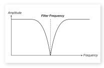
A Notch filter is the opposite of the Band Pass filter, it passes most of the frequencies unaltered, but attenuates those in a specific range.
