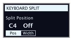
(4) There are two settings for the split point; position and width. Make sure that the Position setting is focused (by pressing the Pos soft button) and set the split point to C4 using the dial.
